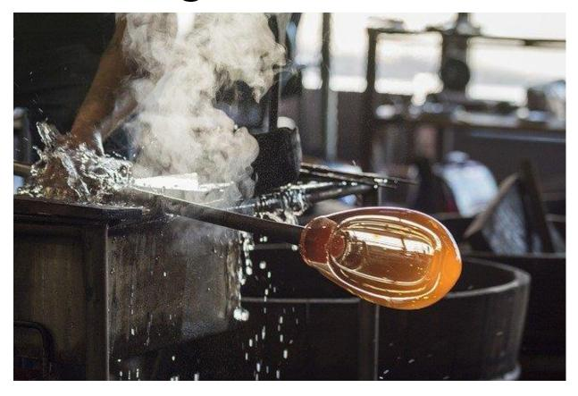
The main ingredient in glass is silica, in the form of sand. When sand is heated to its melting point (around 1700 degrees Celsius), it turns into a liquid, and as it cools, it can be stretched and shaped. Soda ash is added to lower the melting temperature of glass, and limestone is added as a stabilizer. Chemicals and metal compounds can also be added to glass to change properties such as color, opacity, or durability.
